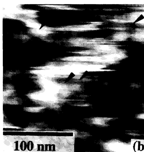
Figure 7 (a) AFM topographic image of SEBS (20/60/20) after large force scanning (central area of 850 \times 850 \text{ nm}^2 ) of 15 nN with the AFM tip. Higher magnification AFM images ( 200 \times 200 \text{ nm}^2 ) (b) of the central area in (a). Typical self-aggregated and stable structures of polystyrene are indicated by arrows in (b)
